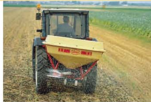
Tramline border spreading with tiltable headstock
