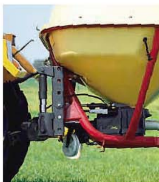
Hydraulically tiltable headstock
