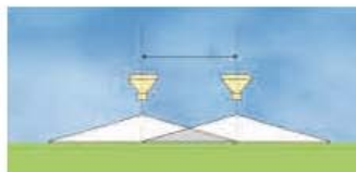
The cone shaped spreading pattern reaches from tractor wheel track to tractor wheel track giving total overlap of the spread surface
