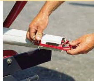
Spout band for 18m spreading width
