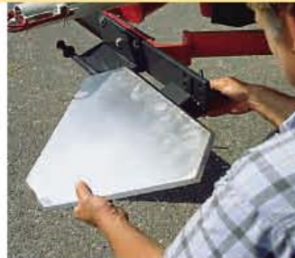
Quick fitting of deflector plates for 18m spreading width
