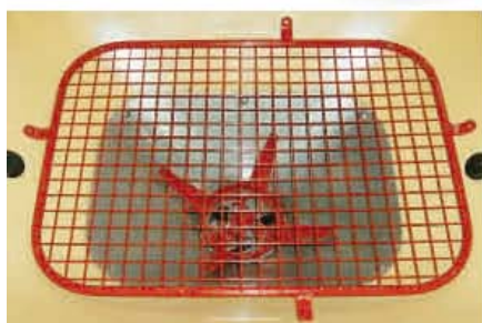
Agitator with safety grid
